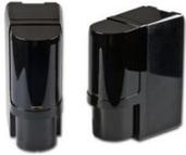
JA-80IR is optical barrier which indicates breach into a protected area by crossing the infra-red line between the transmitter and the receiver. It is a product of company Optex supplemented with transmitters compatible with OASiS system. There can be up to 60m distance between the units. The optical barrier can also be used outdoor, it is protected from dust and water.
