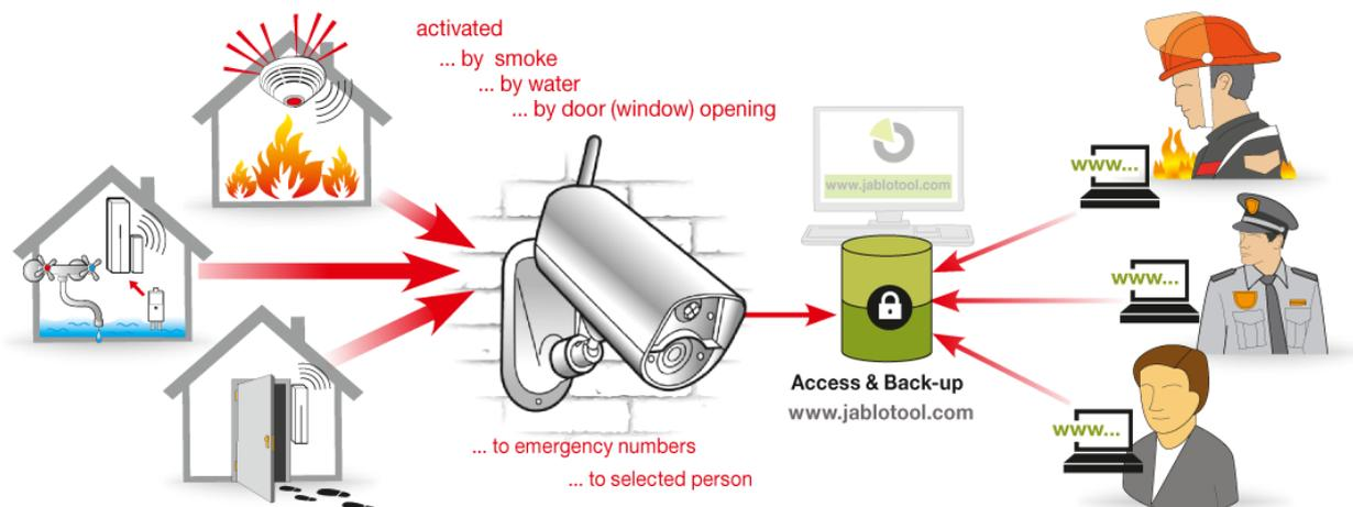
Picture 7: Example of reporting information from detectors via JabloTool application Access & Back-up
