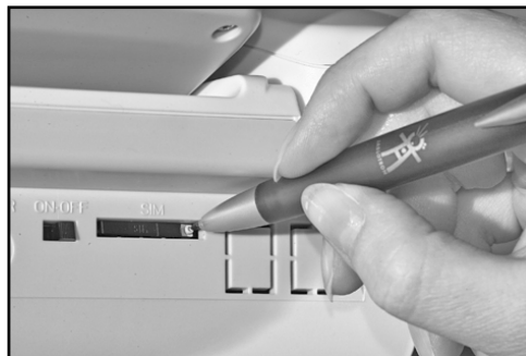
Figure 1: Removing the SIM Card Holder
